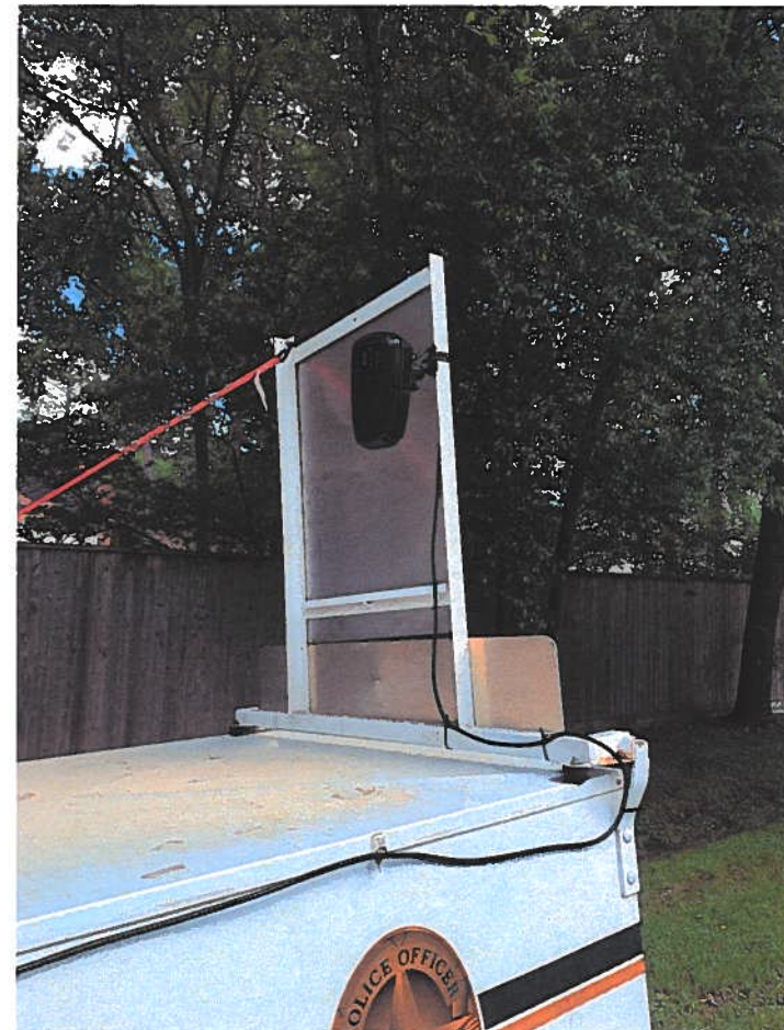
ALPR Installed on the MVPD Radar Trailer Utilizing the Trailer Batteries for Power
