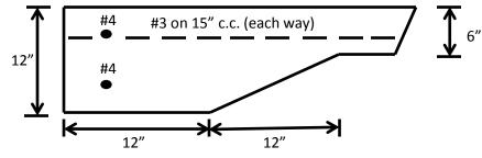
Where the driveway meets the garage slab, install #4 dowels by 24" with plastic sleeve on one end of dowel on 24" centers and additional #4 bar top and bottom of beam.
