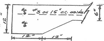
Where the driveway meets the garage slab, install #4 dowels by 24" with plastic sleeve on one end of dowel on 24" centers and additional #4 bar top and bottom of beam.
